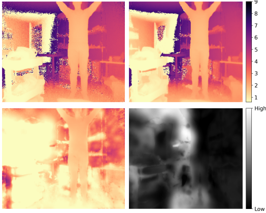
Figure 2. Fitting C-ToF images \neq fitting depth. Top left: Camera-derived depth from C-ToF. Top right: Rendering a GS scene reconstruction into C-ToF raw image samples, then deriving depth. As this is similar to the camera-derived depth to the left, the reconstruction objective was met. Bottom left: Rendered mean scene depth from Gaussians, which is highly inaccurate. Bottom right: Depth distortion error [10], which measures the Gaussian sparsity along each ray. Gaussians are not well localized.
