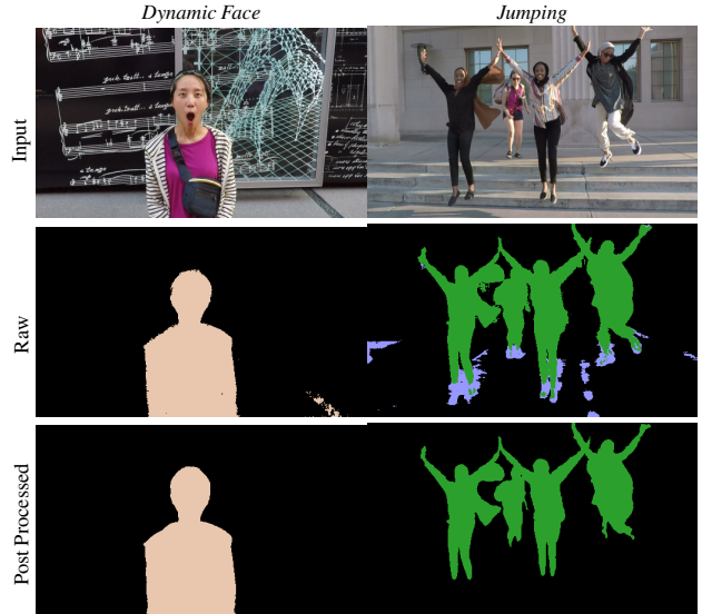
Figure 17: Post processing helps remove small noisy regions from the raw results while maintaining thin features.
